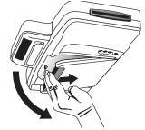
**3** Adjust the angle of the monitor for viewing from the rear car seats.
